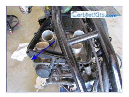
Note: you will notice that there is a hose attached to the front. remove this before completely removing your carburetor assembly. the picture below shows this hose after the carburetor assembly has been removed.
