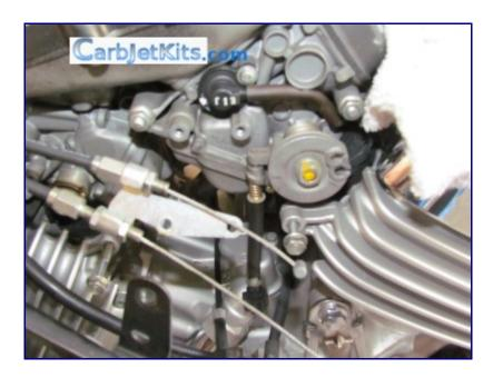
remove the 2 screws that hold the air intake snorkel. there is one on each side.
