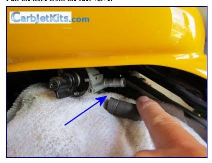
Remove the bolt that holds the gas tank and lift the tank up about 6 inches. Look for the vent hose and remove.
