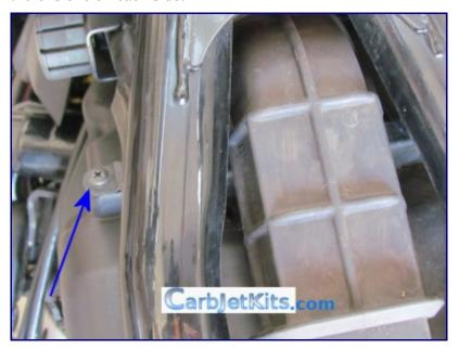
Slide the air intake snorkel towards the back of the bike to remove. When done, it should look like in the picture below.
