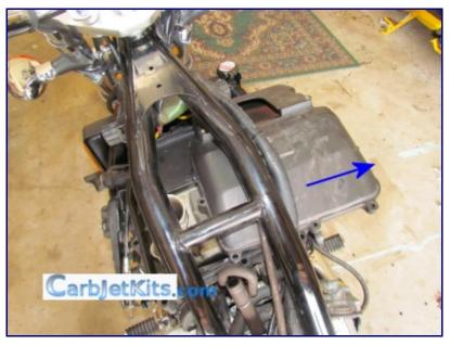
Remove the 3 screws that hold the air filter spacer, but leave the spacer where it is.
