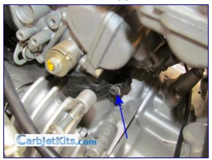
Now the fun part, lift the carburetor bank from the intake spigots.
