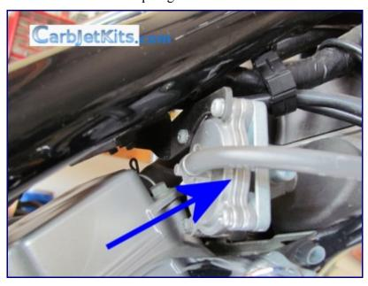
At the top side, remove the 2 bolts that hold the fuel valve diaphragm.
