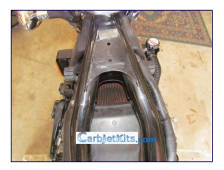
The air cleaner lid is attached with 9 screws.
