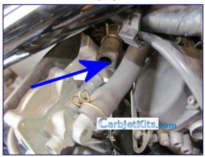
If you not have done so, remove both plastic side covers. at the thermostat housing (right side) remove the bolt as shown in the picture below.
