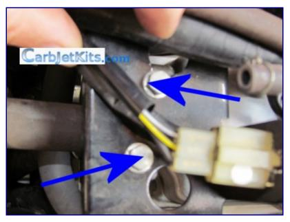
Note: you only have to remove the left bolt completely and loosen the right bolt.
